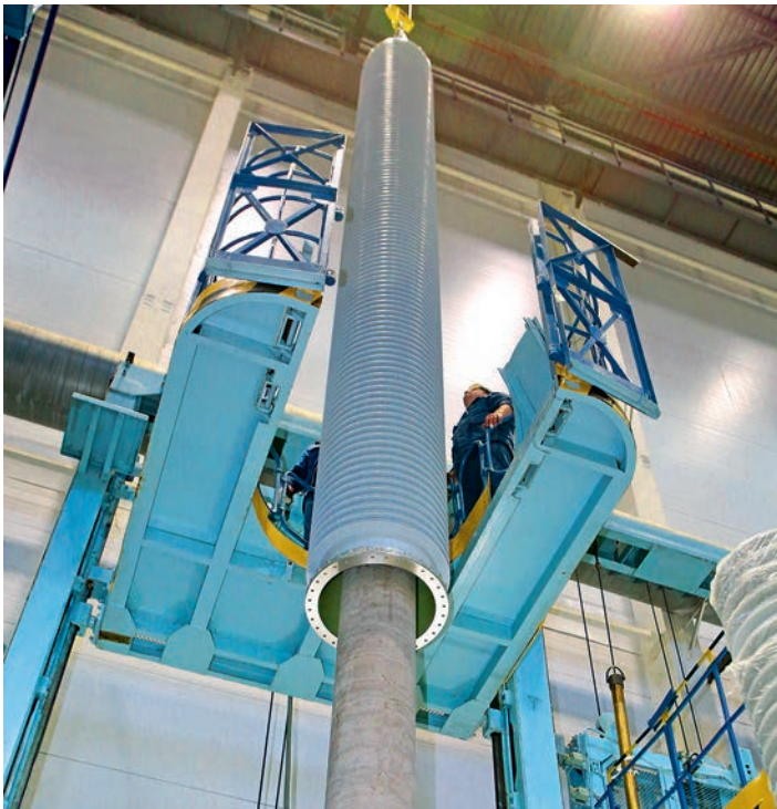
Installation of external insulation of the bushing — composite housing
