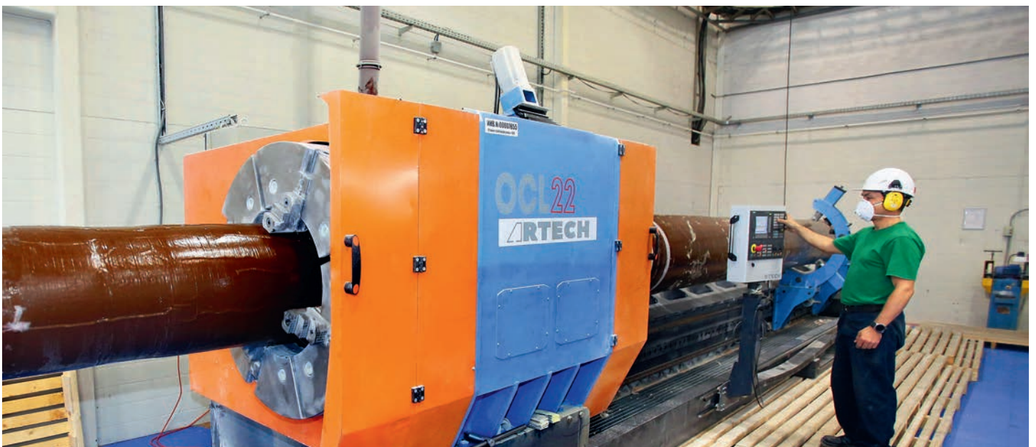
Machining of the internal insulation of the 1200 kV bushing on a lathe with numerical control to give the insulation the required geometry
