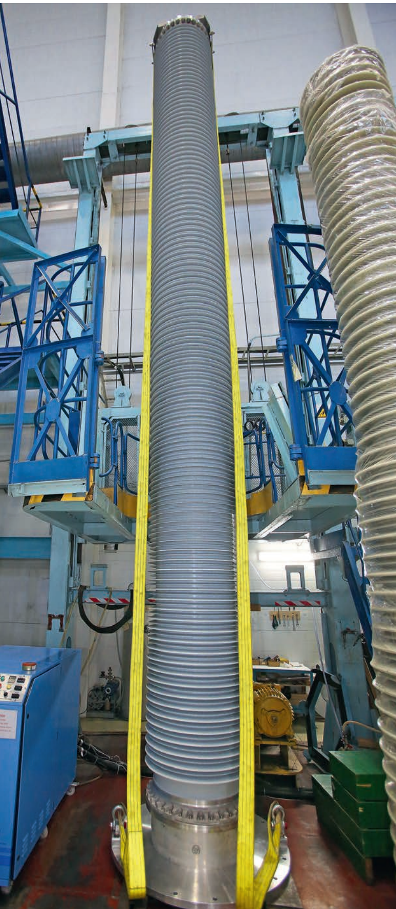
Filling the bushing's cavity with a dry filler — compression gel
