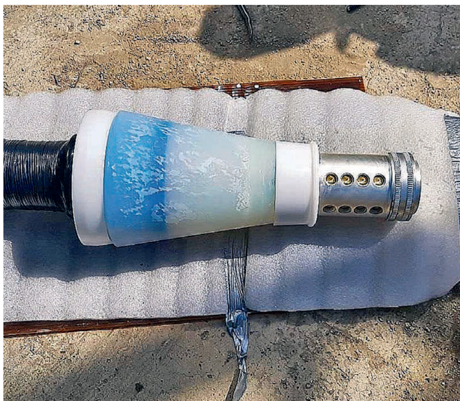
Izolyator-AKS IKV-252 cable connector during testing
