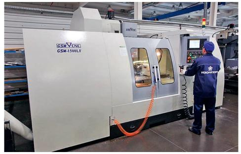
CNC Vertical Milling Center GSM-1500LF
