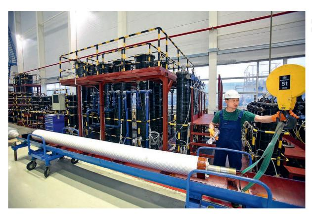
■ The core impregnation – key process operation in the production of a bushing
