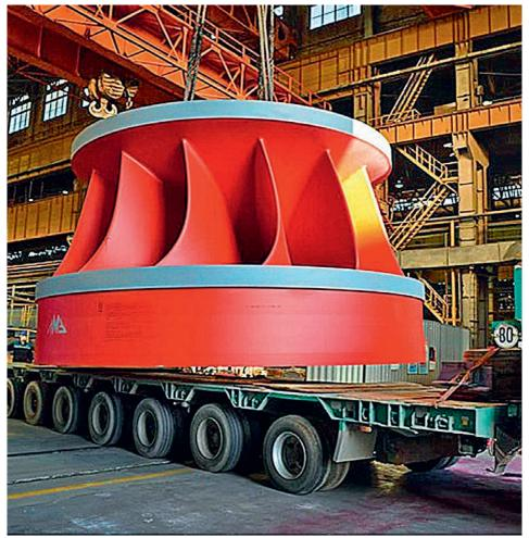
Shipment of a hydraulic turbine runner for the Ust-Srednekanskaya HPP, manufactured at the Leningrad Metal Plant of Power Machines (photo: Power Machines)
