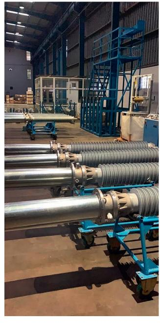
▼ Loading bushings for delivery to the transformer plant Transformers & Rectifiers (India) Limited
