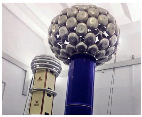
The state primary special standard of the unit of direct current electrical voltage, which has passed improvement - volt in the range of  $\pm$  (1 . . . 500) kV (photo: VNIIMS)
