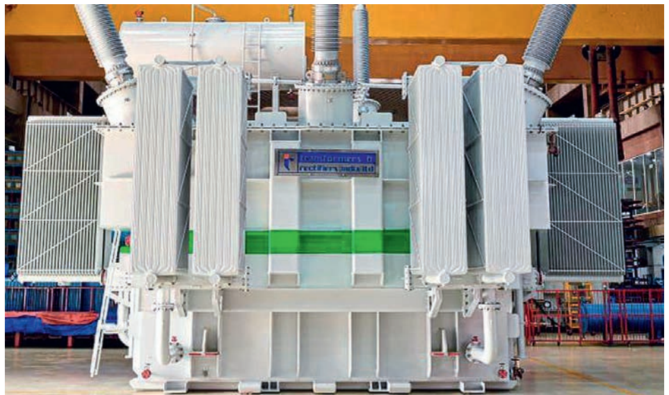
T&R three-phase shunt reactor 420 kV, 50 MVAR filled with liquid ether dielectric equipped with Izolyator bushings
