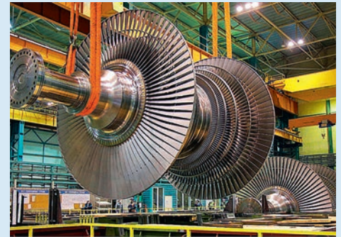
Assembling the prototype of the first low-speed turbine with a capacity of over 1250 MW at the Leningrad Metal Plant, a part of the Power Machines company (photo: Power Machines)
