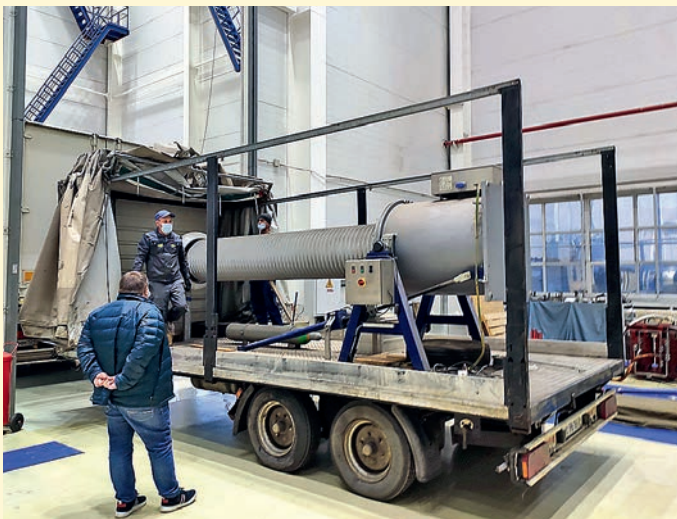
A reference mobile voltage transformer 500 kV delivered to the test center of Izolyator plant under an agreement with the All-Russian Research Institute of Metrological Service
