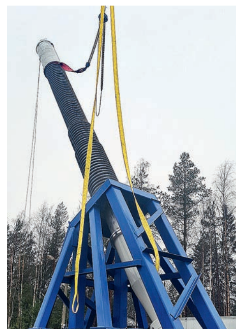
A 750 kV Izolyator transformer bushing on the seismic platform of the Center for Complex Seismic Testing in the Leningrad Region
