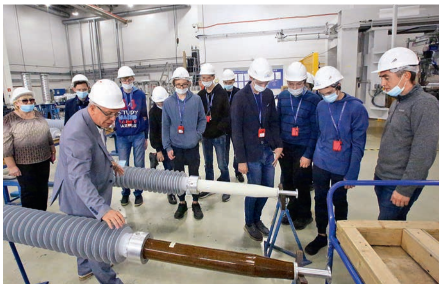
Students of the Krasnogorsk College are getting familiar with the design and production stages of high-voltage bushings
