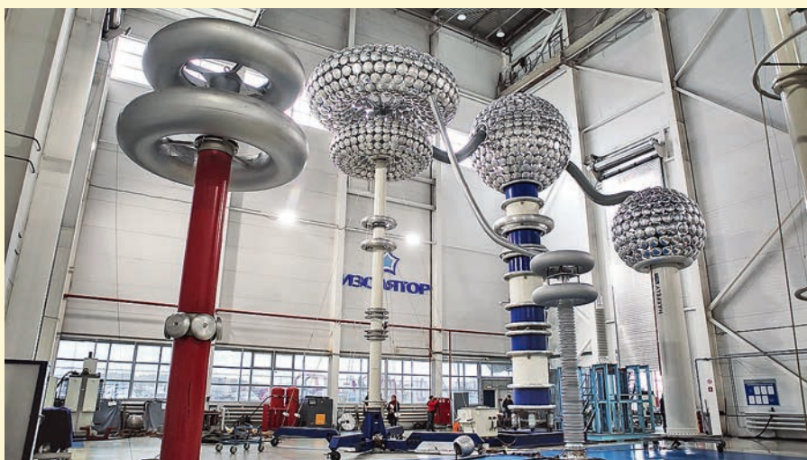
Testing of bushing under operating voltage of 420 kV prior to shipment
