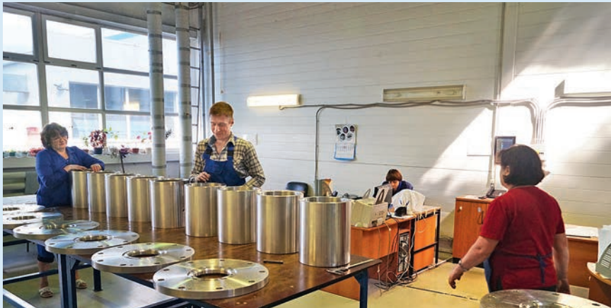
Entry quality control of purchased components of high-voltage bushings by the quality service of the Izolyator plant
