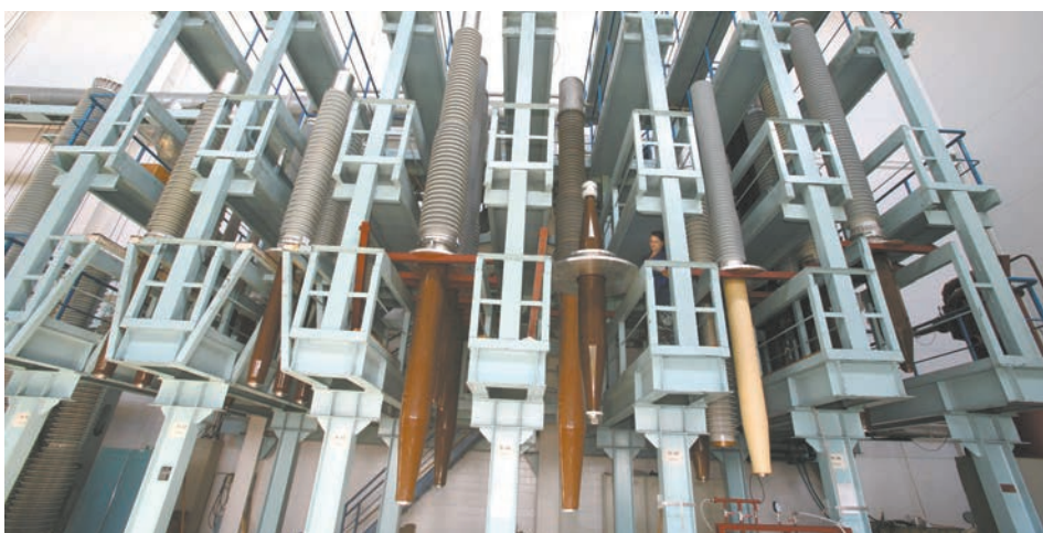
High-voltage bushings seated on racks at the assembly shop at Izolyator plant
