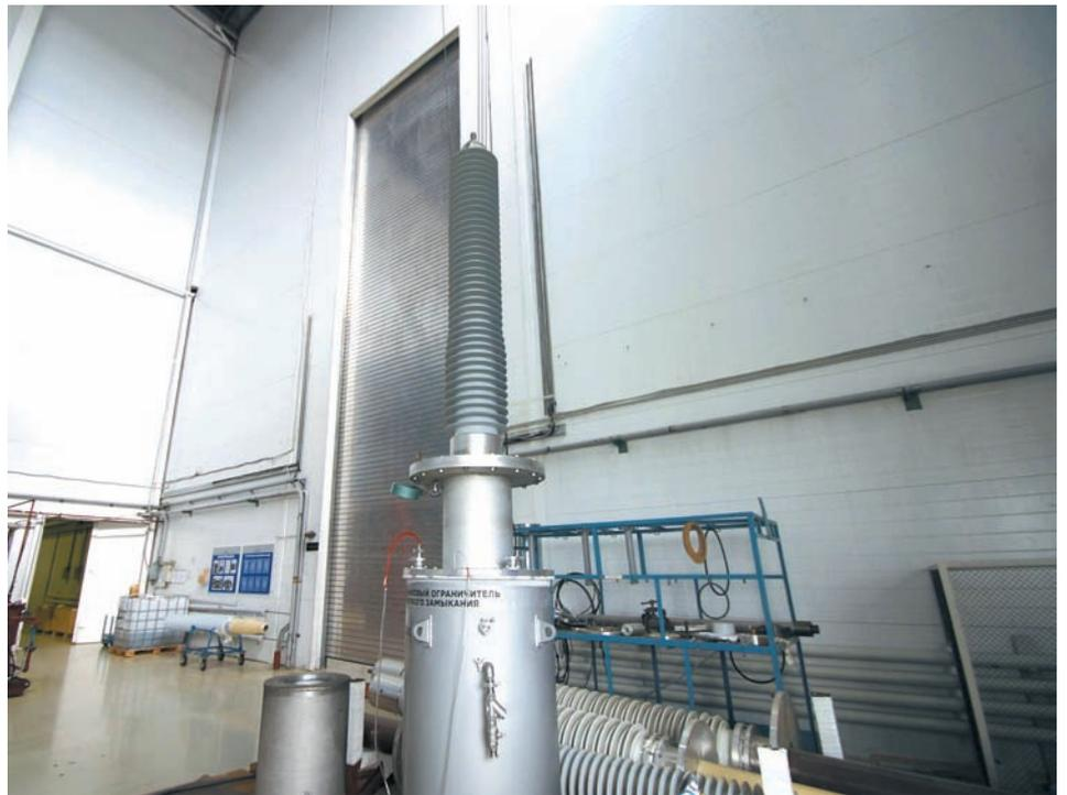
220 kV air-liquid nitrogen bushing tests at  $-200^{\circ}\text{C}$
