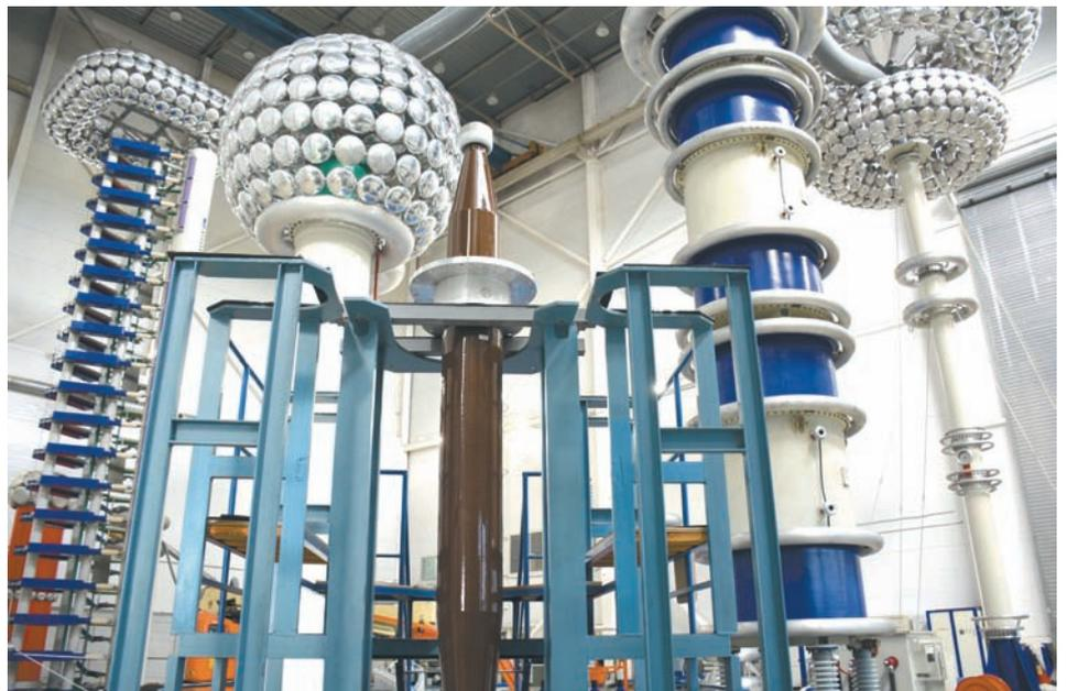
*500 kV oil-SF6 gas bushing tests at Izolyator plant*
