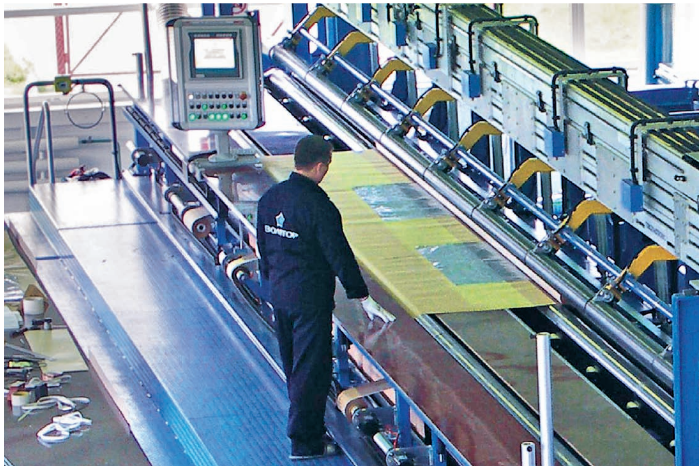
Paper core winding machine up to 12 m
