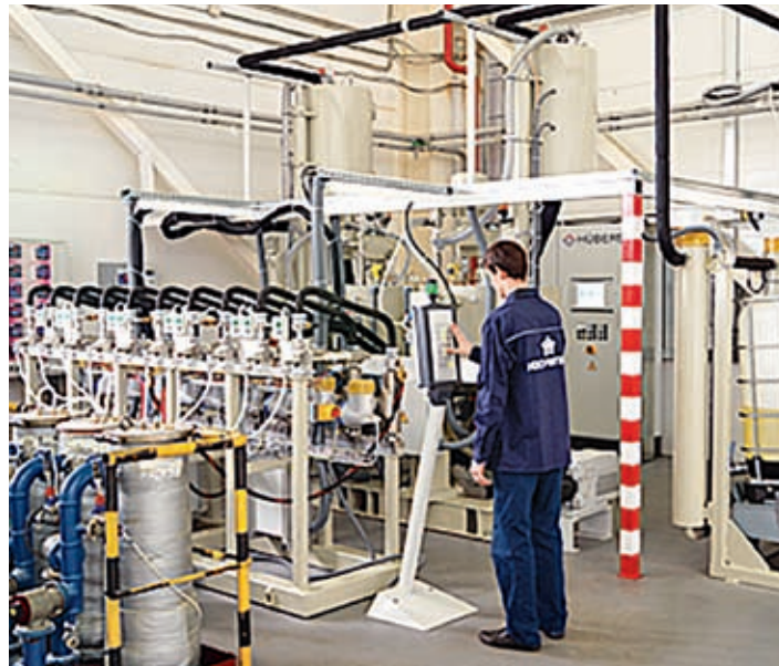
Airvoid mixing and dosing Hübers unit at Izolyator plant
