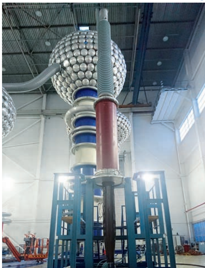
500 kV oil-SF6 bushing's tests at Izolyator plant
