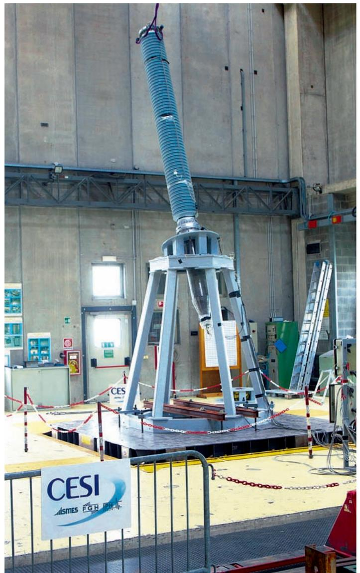
*Seismic tests in progress*
