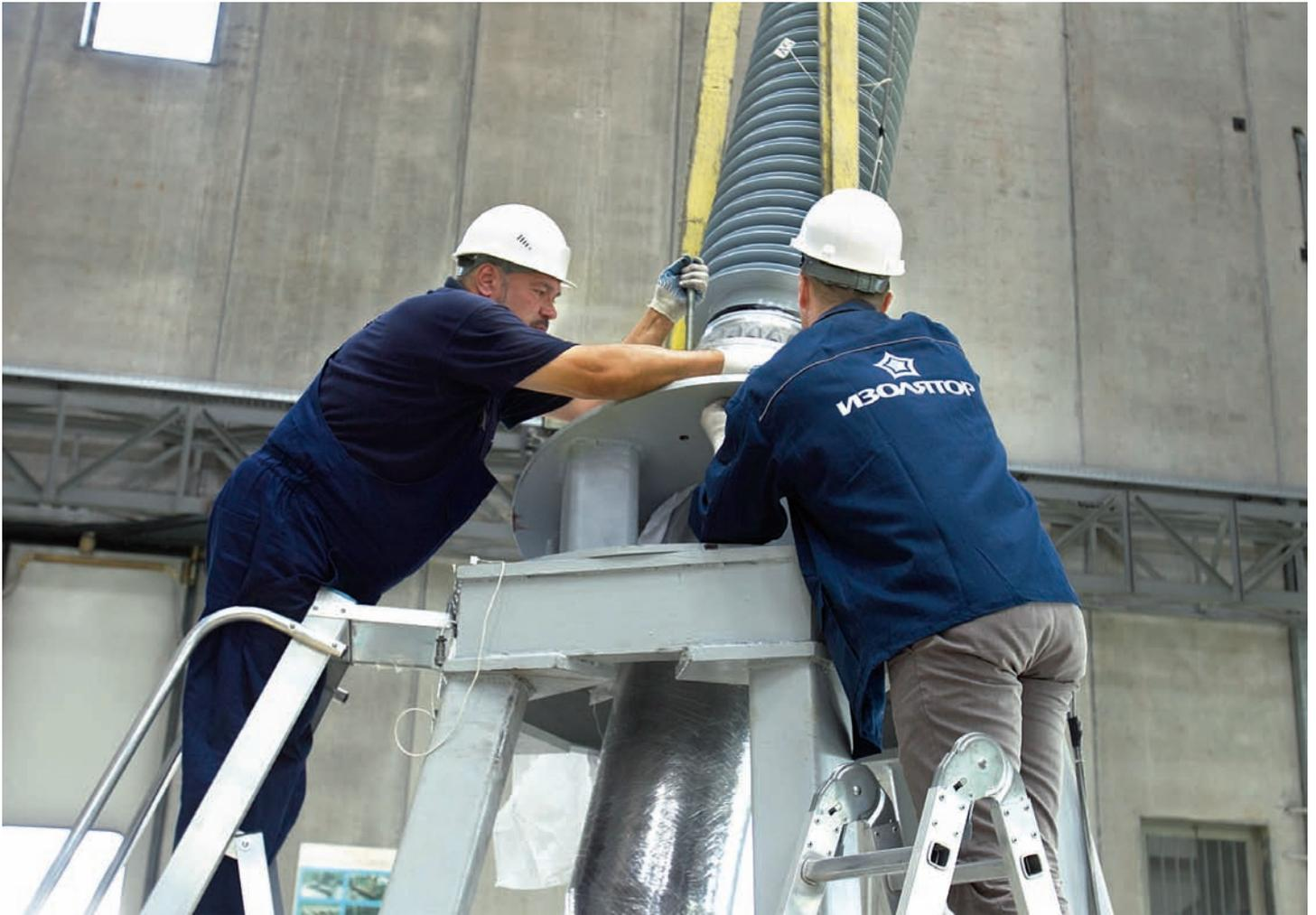
*Installation of a bushing on a test rack*
