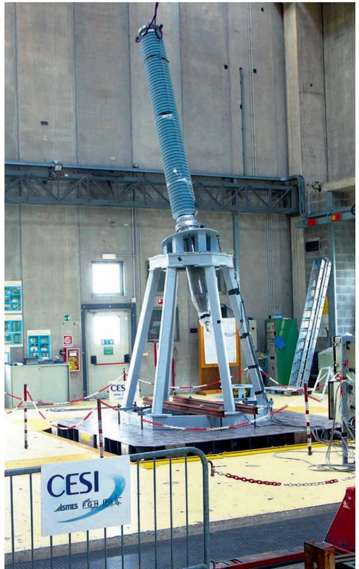
*Seismic tests in progress*
