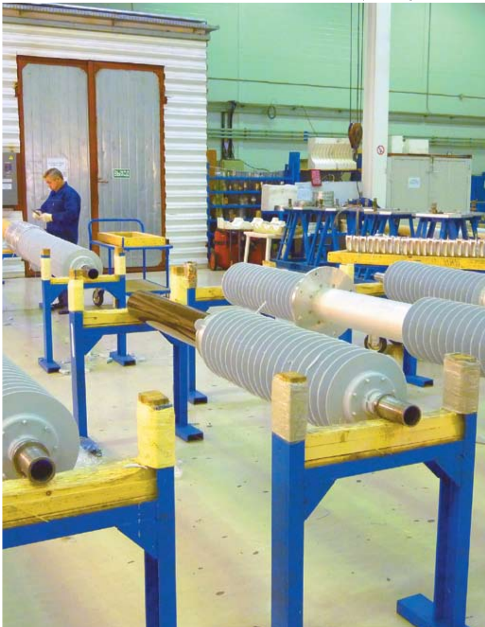
110 kV Izolyator bushings with RIP insulation
