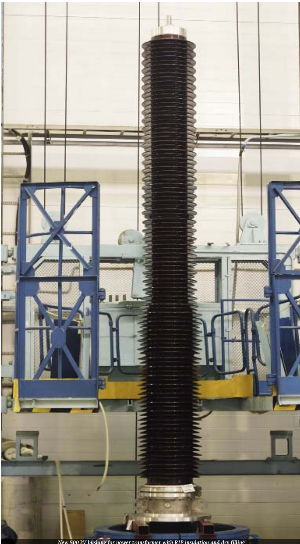
New 500 kV bushing for power transformer with RIP insulation and dry filling
