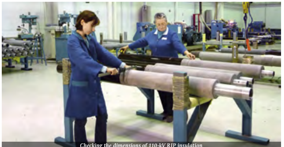
Checking the dimensions of 110-kV RIP insulation
