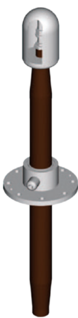
Oil to Oil Bushings for cable connection to transformer Voltage: 110–500 kV, Current: 630–1000 A
